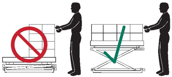
As the load is added and removed from the pallet, the height of the platform will raise or lower to maintain the proper working height. To adjust the working height, add or remove air from the system.
