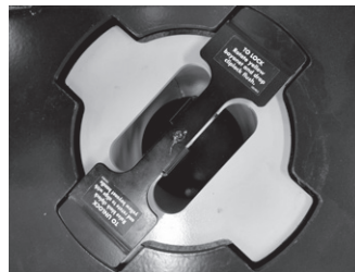
INITIAL BAYONET POSITION IN PLATFORM
