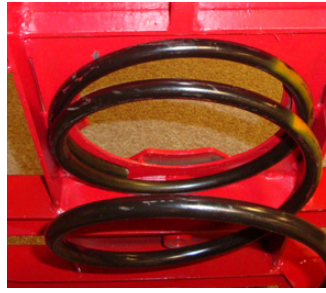
ORANGE SPRING PROPERLY POSITIONED IN UPPER POCKET
