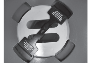
TURN CLIPLOCK 45 DEGREES CCW AND LOWER TO LOCK
