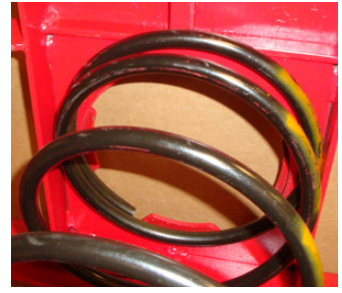
ORANGE SPRING IMPROPERLY POSITIONED IN UPPER POCKET
