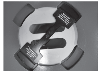
TURN CLIPLOCK 45 DEGREES CCW AND LOWER TO LOCK
