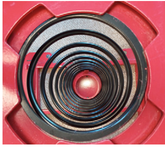
WHITE SPRING IMPROPERLY POSITIONED IN UPPER POCKET
