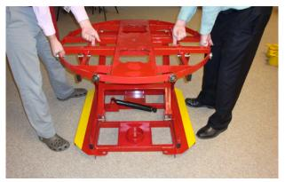
4. Lift the latch stops and hold them up. Continue to lift the platform until it reaches its fully raised position.
