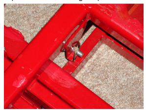
12. Reinstall the yellow bayonet(s) by inserting them into the bayonet openings and turning them clockwise into the locked position. Secure with the black clip locks.
