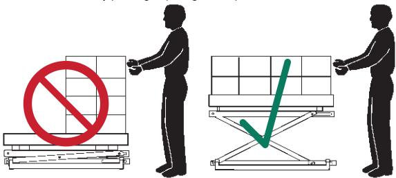
When manually unloading, always unload the pallet uniformly in even layers. As the pallet is unloaded the platform will raise, maintaining the proper working height in the ergonomic range. Do not reach over the load. Instead rotate the load by pushing or pulling on the pallet.
