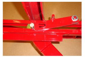
13. Reinstall the dampener and secure with the pin.
