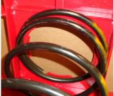
ORANGE SPRING IMPROPERLY POSITIONED IN UPPER POCKET
