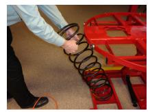
9. While one person holds the platform up the second person removes the dampener pin from the hole in the roller track nearest to the hinge end.
