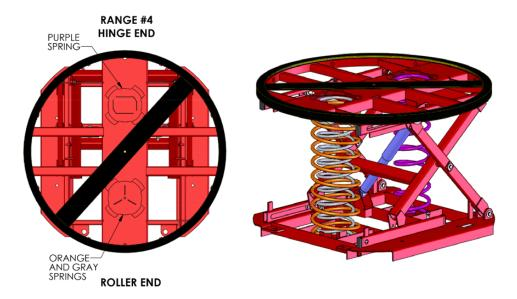
3. After appropriate spring(s) are in place, install the yellow bayonet(s) by inserting them into the bayonet openings and turning them clockwise into the locked position. Secure with the black clip locks.
