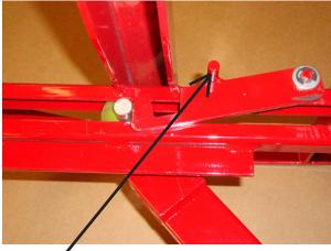
RELEASE LATCH STOP BY PULLING UP HERE (BOTH SIDES)
