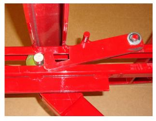
5. While one person holds the platform up the second person places the dampener pin into the hole in the roller track nearest to the hinge end to hold the platform in place.
