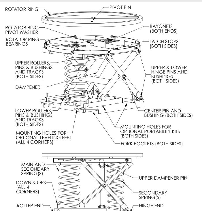
Note: The rotator ring may be ordered as a solid round or rectangular top, or ordered with a locking device. The rotator ring may also not be included at all.
