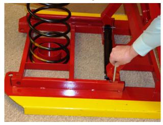
6. Remove the bayonets by lifting the cliplock and turning 45 degrees CW, then turning the bayonet 45 degrees CCW and lifting out. Place the bayonets aside in a safe location.
