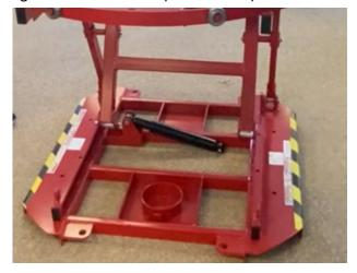
6. Remove the roller end bayonet by lifting the cliplock and turning 45 degrees CW, then turning the bayonet 45 degrees CCW and lift out. Place the bayonet aside in a safe location.
