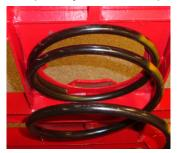
ORANGE SPRING PROPERLY POSITIONED IN UPPER POCKET
