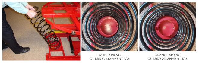
8. Grasp the spring by the second or third coil down from the top, compress the spring and slide the top of the spring into the upper spring pocket.
