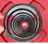
WHITE SPRING IMPROPERLY POSITIONED IN UPPER POCKET
