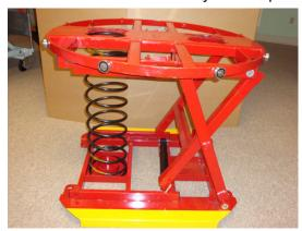
12. Press down on the platform until the two latches fall into place. The latches will fall in behind the roller pins.
