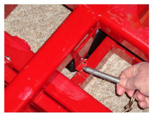
3. With two people, lift the platform until the roller pins contact the upper latch stops located on the platform on both sides.
