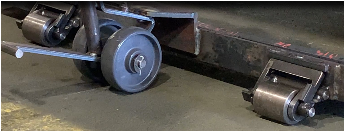
Flip Down Wheels in Latched Position, Dolly Jack Engaged
