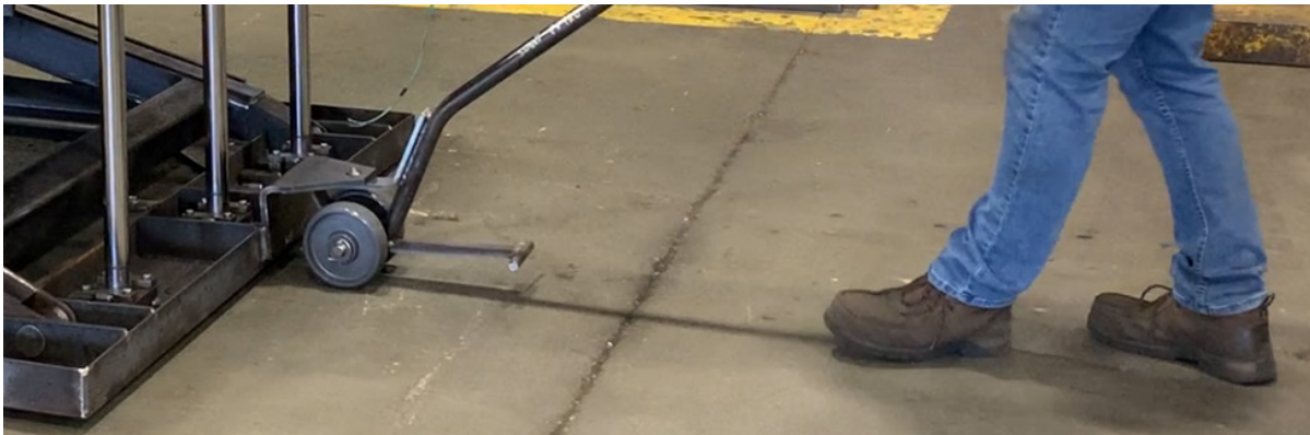
Dolly Jack Engaged, Flip Wheels in Latched Position, and Ready to Relocate
