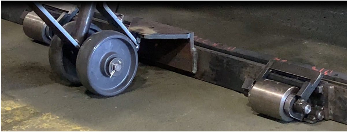
Flip Down Wheels in Storage Position, Dolly Jack Not Yet Engaged
