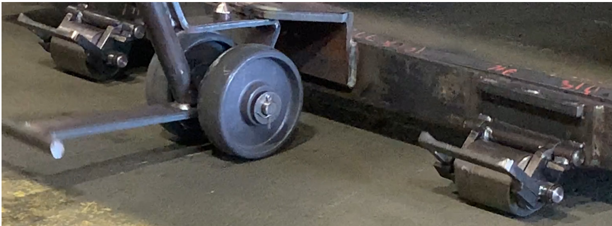
Flip Down Wheels in Free Position, Base Frame Raised, Dolly Jack Engaged (Once base frame is lowered to floor, Flip Down Wheels will rotate up to Storage Position)
