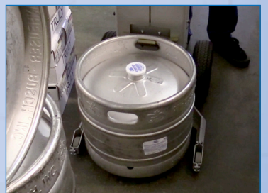
Adjustable lifting bracket accommodates shorter kegs
